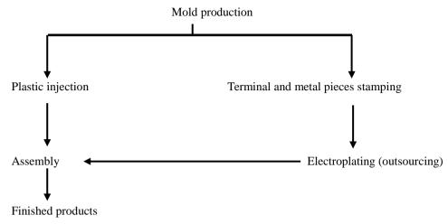
There are 5 major stages in the production process of connectors, which are mold development, plastic injection, stamping, electroplating, and assembly. Currently, the Company outsources for electroplating after the design and the works of all other stages of the process are performed by its own technologies. The Company has accomplished the vertical integration of 5 major processes in 2012 for the realization of all-indigenous production plan.
